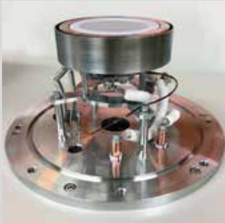
Φ4inch_1200C, SiC coated heater
