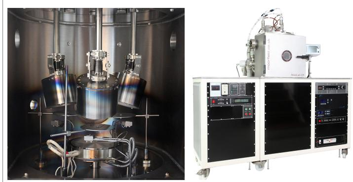
Left: MiniLab 125 chamber interior, with 3 magnetron sputtering sources for 4" diameter targets arranged in a sputter-down configuration. At the bottom of the chamber is a 1000 °C substrate heating stage with bias, quartz crystal sensor heads for deposition rate/thickness control and various shutters. Right: MiniLab 125 system with extended control rack. System is configured for magnetron sputtering and is equipped with automatic process control.
