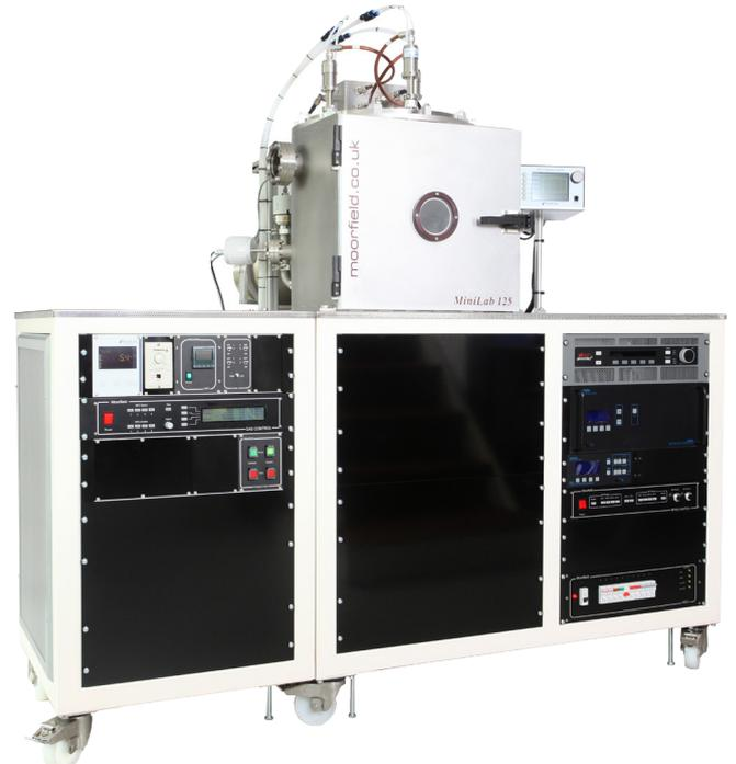
Left: MiniLab 125 chamber interior, with 3 magnetron sputtering sources for 4" diameter targets arranged in a sputter-down configuration. At the bottom of the chamber is a 1000 °C substrate heating stage with bias, quartz crystal sensor heads for deposition rate/thickness control and various shutters. Right: MiniLab 125 system with extended control rack. System is configured for magnetron sputtering and is equipped with automatic process control.
