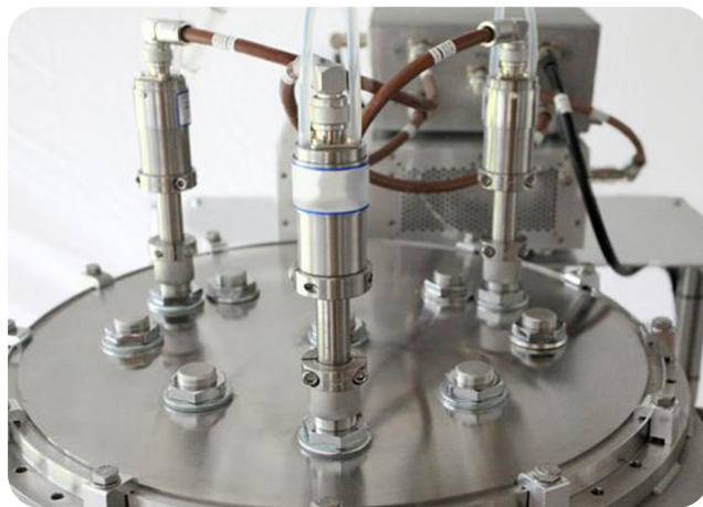
Minilab 125 chamber roof, with removable top-plate allowing for future re-configuration
